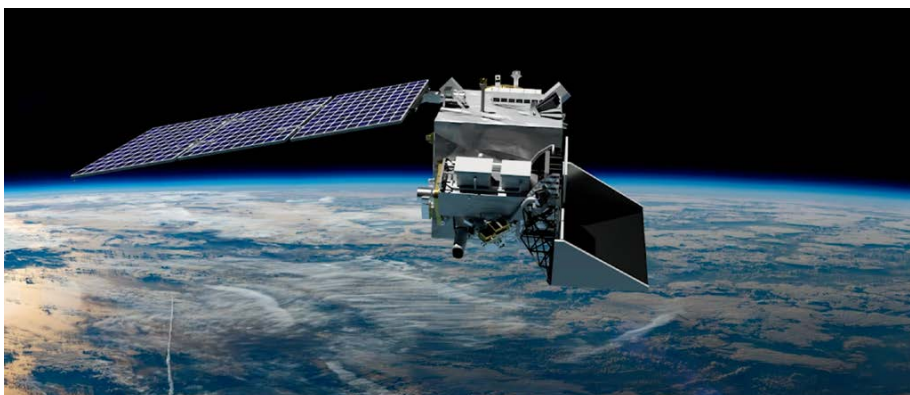
FIGURE 1. A rendering of the PACE spacecraft. Three instruments will fly on board: a hyperspectral imager and two multi-angle polarimeters. Credit: NASA Conceptual Image Laboratory, https://svs.gsfc.nasa.gov/12469
