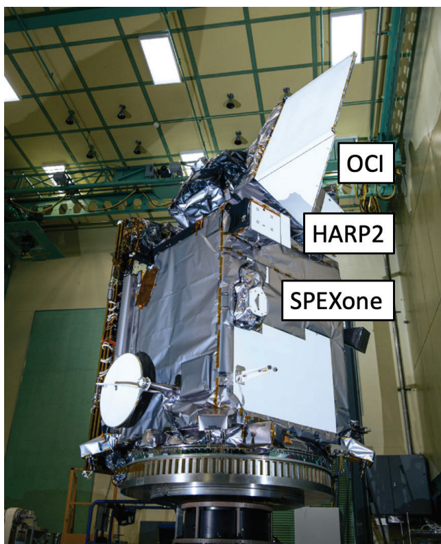
The full PACE observatory with OCI, HARP2, and SPEXone all indicated. Credit: Dennis Henry| NASA GSFC
