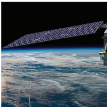
An array of solar panels are needed to power PACE. Before launch, the solar array is folded and then unfurls in orbit. For this model, the **Beam** is a single piece that connects the **Solar Array** to the **Bus**.
