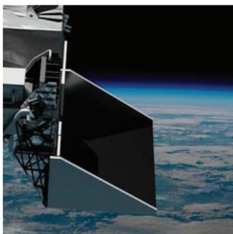
A **Radiator Shield** blocks out nearly 80% of Earth’s energy.
