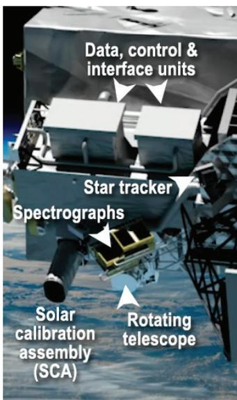
*The Ocean Color Instrument (OCI) is designed to measure light at finer wavelength resolution than previous NASA sensors. Its spectrographs will split light down to 5 nanometers (5 one-billionths of a meter)!*
