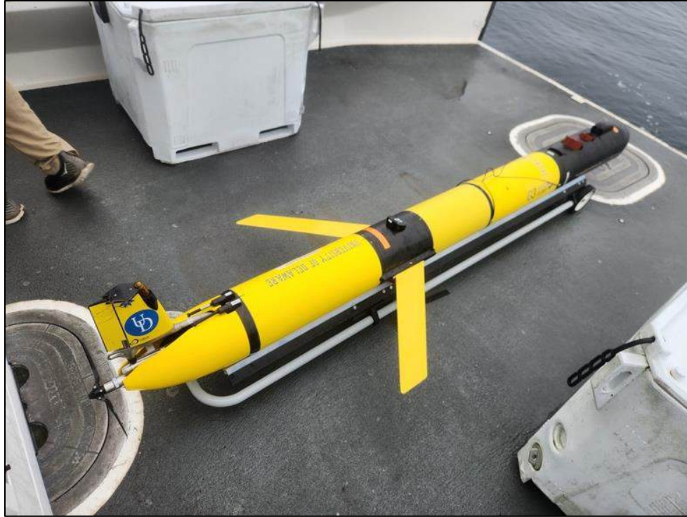
Figure 36 Orris after recovery during PACE-PAX. The forward upward looking transducers are the WBAT-mini. The mid-section has the upward looking irradiance sensors. Under glider are the downward looking radiance sensors, CTD, and ECO-Triplet.
