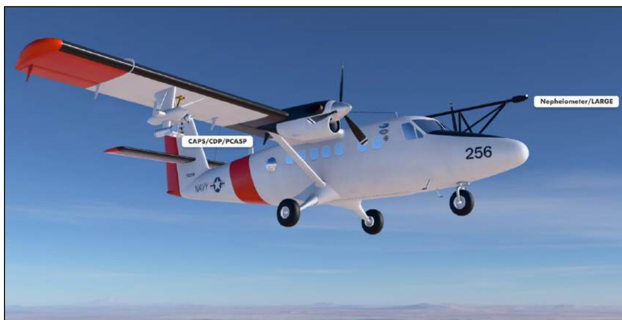
Figure 20 Rendering of the NPS CIRPAS Twin Otter, with indicated instrument inlet placement. Renderings available at https://airbornescience.nasa.gov/3d-models .
