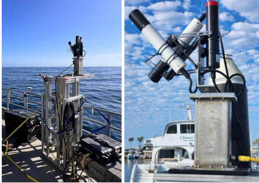
Figure 17 PySAS above-water radiometry system measuring (1) water-leaving (upwelling) radiance, (2) sky radiance and (3) downwelling solar irradiance, which are used to derive aquatic remote sensing reflectance ( R_{rs} ), the most fundamental ocean color data product from which all other products are derived.
