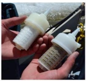
Spectral Backscatter Sensor (472, 526, and 654 nm)
